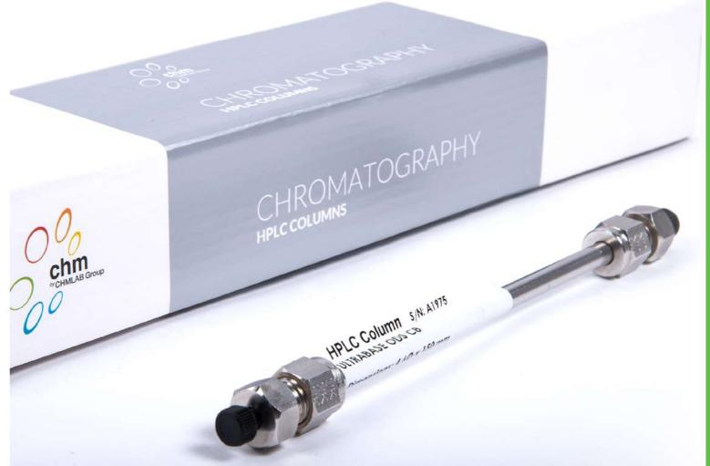
The ULTRABASE® silica has high chemical purity; its metal ion content of Fe, Zr, Al and Ti is <10~ppm
